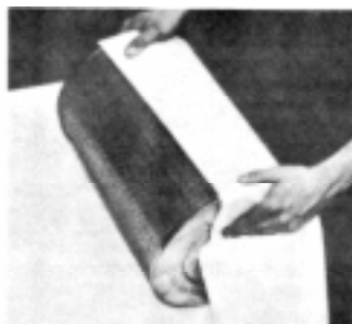
2. Wrap and store good Elements in a clean dry place.
