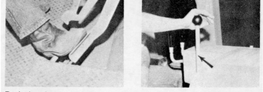
Push decelerator to override governor control and reduce engine speed Release decelerator to increase engine speed to governor control setting.
